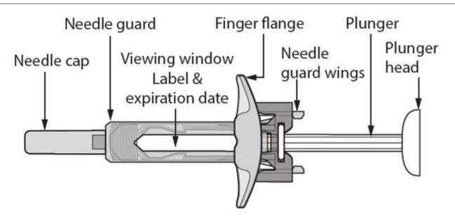
**Figure A**: HYRIMOZ prefilled syringe with BD UltraSafe Passive  $^{\text{\tiny{M}}}$  Needle Guard and finger flange
