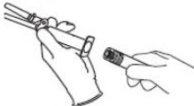
**DO NOT PUSH VIAL INTO INJECTOR; THIS MAY CAUSE MISALIGNMENT OF THE INJECTOR NEEDLE.**
