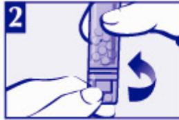
2 Twist until 5 pellets are dispensed into cap.
