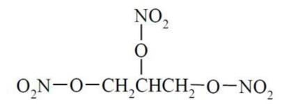
C<sub>3</sub>H<sub>5</sub>N<sub>3</sub>O<sub>9</sub> Molecular weight: 227.09
