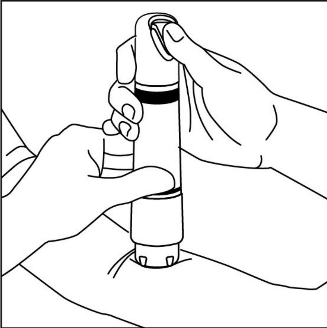
Ensure that the patient's treatment site is supported to prevent movement. Seal the purple ZINGO outlet against the patient's skin. Hold the device perpendicular to the skin, making sure that your thumb can reach the green start button.
