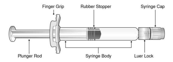
**Step 1:** Holding the Luer lock in one hand (avoid holding the plunger rod or syringe body), unscrew the syringe cap by twisting it counter-clockwise with the other hand.
