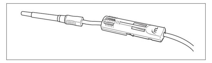
2. Ensure that the three lock points on the DonorCare are locked closed.
