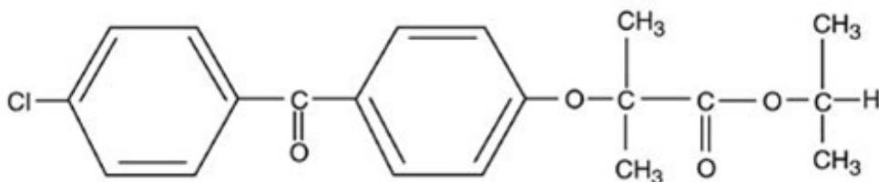
The empirical formula is C<sub>20</sub>H<sub>21</sub>O<sub>4</sub>Cl and the molecular weight is 360.83; fenofibrate is insoluble in water. The melting point is 79 to 82°C. Fenofibrate is a white solid which is stable under ordinary conditions.
