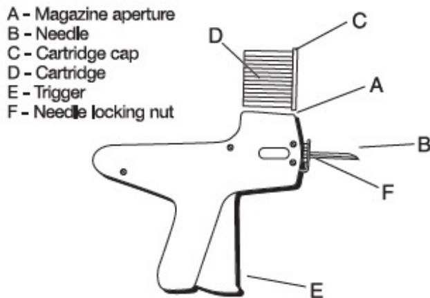
Fig. 3 - Diagram of the Implanter and Cartridge
