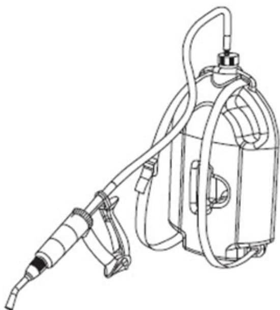
Figure 2. 5L bottle and applicator device with tubing.
