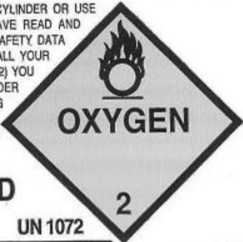
**OXYGEN, U.S.P. PRODUCED BY AIR LIQUEFACTION. WARNING: HIGH PRESSURE OXIDIZING GAS. VIGOROUSLY ACCELERATES COMBUSTION.** Secure cylinder in storage and use. Keep oil and grease away. No smoking in cylinder area. Open valve slowly. Use only with equipment cleaned for oxygen service and rated for cylinder pressure. Close valve after each use and when empty. Use in accordance with Material Safety Data Sheet.
