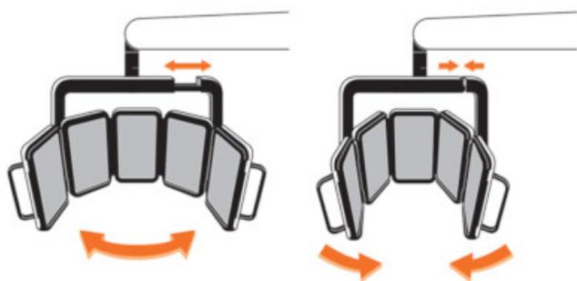
**Figure 5:** Movement range of the lamp head.
