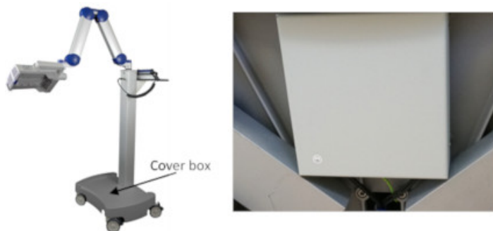
Figure 23: BF-RhodoLED®. (The appearance of devices from batches 001 to 003 slightly differs. Appearance and location of the labels remain unaltered.)
