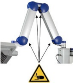
Figure 1: The scissor arm in parked position. Arrows indicate potential points where fingers can get trapped. (The appearance of devices from batches 001 to 003 slightly differs. Appearance and location of the labels remain unaltered).
