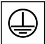
Figure 23: Instruction for ground connector connection (not visible from the outside)
