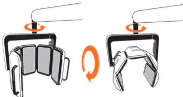
**Figure 4:** Rotation and tilting of the lamp head.
