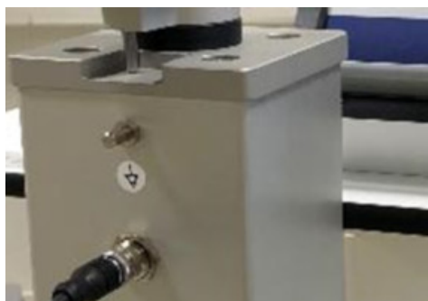
Figure 24: Potential compensator conductor. (The appearance of devices from batches 001 to 003 slightly differs. Appearance and location of the labels remain unaltered.)
