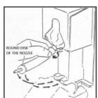
4. Before closing the cover, check to make sure the round disc of the nozzle is firmly in place at the bottom of the lower locator.
