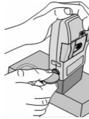
4. Insert a coin into the slot in the cassette latch, push in, and turn counterclockwise until the line on the latch lines up with the arrow on the side of the pump and you feel the latch click into place.
