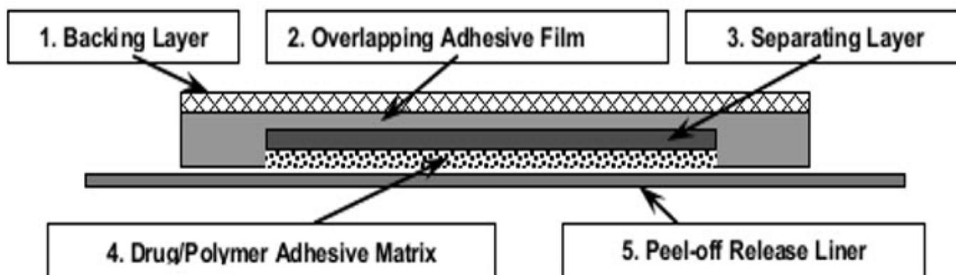
**Figure 1: Cross-Section Diagram of BUTRANS (not to scale).**
