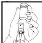
Step 2. Hold the container upright and facing away from yourself and others. Press down on the top of the grooved button 5 times. (See Figure C)
