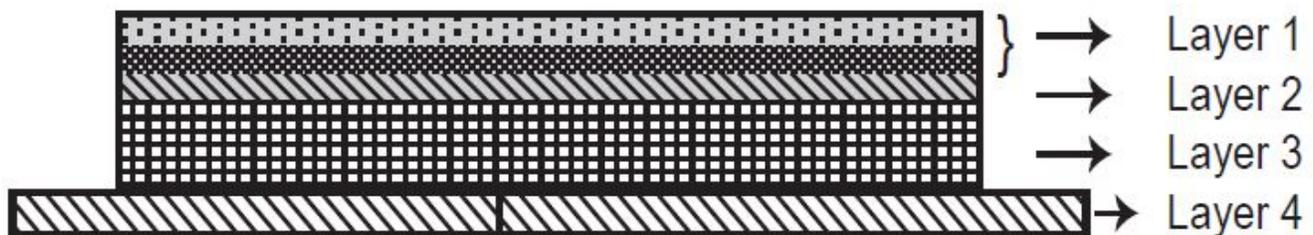
Layer 1: Copolymer foam backing with adhesive layer
