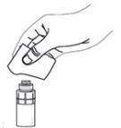
After cleaning, wait for about 1 minute to allow the valve to dry.
