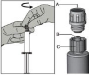
6. Pull the cap (A) off in a straight upward direction. DO NOT TOUCH THE STERILE SYRINGE TIP (Luer-Lok) (B) (see Figure 2).
