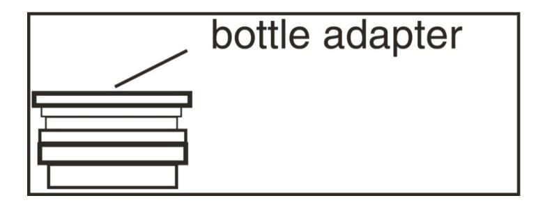
Once the bottle adapter is installed, it cannot be removed. See Figure D.
