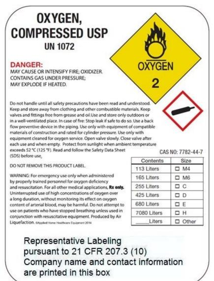
OXYGEN COMPRESSED USP UN 1072 DANGER: MAY CAUSE OR INTENSIFY FIRE; OXIDIZER. CONTAINS GAS UNDER PRESSURE; MAY EXPLODE IF HEATED.
