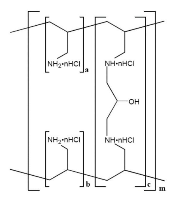
a, b = number of primary amine groups a + b = 9 c = number of crosslinking groups <math>c = 1 n = fraction of protonated amines <math>n = 0.4 m = large number to indicate extended polymer network
