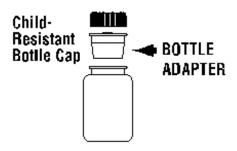
2. Close the bottle tightly with cap. This will assure the proper seating of the bottle adapter in the bottle
