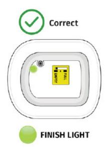
Check to see if the status light is **SOLID GREEN** or has switched off. This means the dose is complete.
