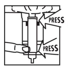
Align the half moon ears (round side out) with the slots of the dispenser's lower docking area. Press top and bottom of tube firmly into place.
