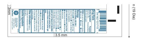
Key Line Drawing for Seamless Printed Tubes Dia 25, Tube Length 125 mm With Topseal and Screw on Cap Orifice 4mm
