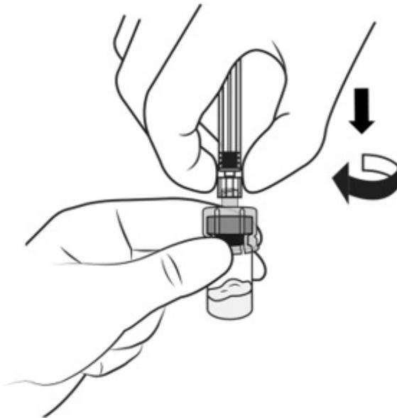
(b) Maintaining your grip on the spin lock, attach the syringe to the vial adapter by screwing the spin lock clockwise onto the vial adapter luer lock. ***Gently twist the spin lock until it stops turning to ensure a tight connection.***
