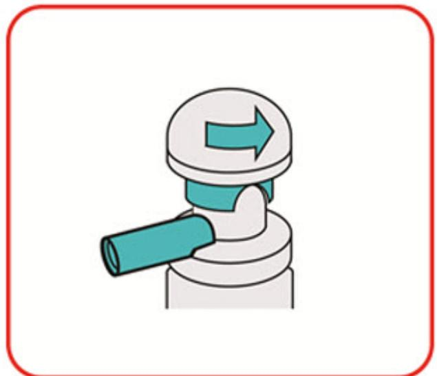
**Step 11: Twist Notch on Dome Away from Nozzle**
