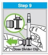
Holding onto the sprayer body, pinch and remove the dose divider clip from plunger.
