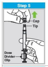
Hold on to the sprayer body and pull off the gray cap.
