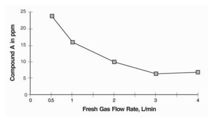
Since the reaction of carbon dioxide with absorbents is exothermic, the temperature increase will be determined by quantities of CO  $_2$ absorbed, which in turn will depend on fresh gas flow in the anesthesia circle system, metabolic status of the patient, and ventilation. The relationship of temperature produced by varying levels of CO  $_2$ and Compound A production is illustrated in the following in vitro simulation where CO  $_2$ was added to a circle absorber system.
