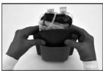
Hold the bundle and insert into the centrifuge cup.
