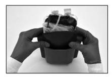
6 Hold the bundle and insert into the centrifuge cup.
