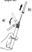
Align vial such that the injector needle is centered on the stopper.
