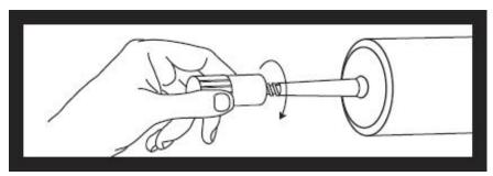
Attach luer locknut to syringe by holding dust cover and screwing to the stop.
