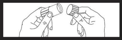
Next remove cap from luer locknut dust cover by twisting to break tamper evident seal. Discard cap.
