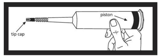
Remove syringe from carton and inspect the area around the **tip cap** and outside of **piston** for signs of leakage. Do not use if leakage is observed. Load syringe into power injector.
