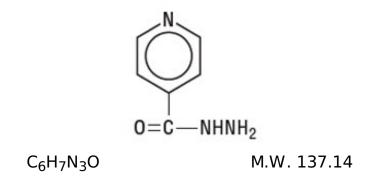
Isoniazid, USP is odorless, and occurs as a colorless or white crystalline powder or as white crystals. It is freely soluble in water, sparingly soluble in alcohol and slightly soluble in chloroform and in ether. Isoniazid, USP is slowly affected by exposure to air and light.
