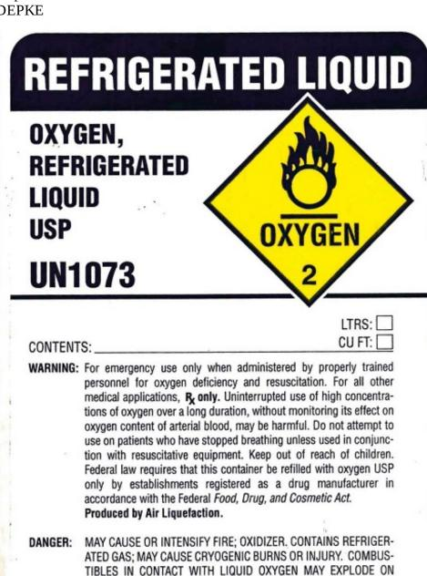
IGNITION OR IMPACT. Do not handle until all safety precautions have been read and understood. Keep and store away from clothing and other combustible materials. Keep valves and fittings free from grease and oil. Use and store only outdoors or in a well-ventilated place. Wear cold insulating gloves, face shield, and eye protection. In case of fire: Stop leak if safe to do so. Use a back flow preventive device in the piping. Use only with equipment of compatible materials
