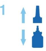
Remove spray nozzle by grasping at base and pulling up.
