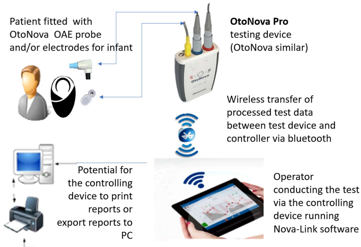
Figure 2. Operation of the OtoNova with Nova-Link
