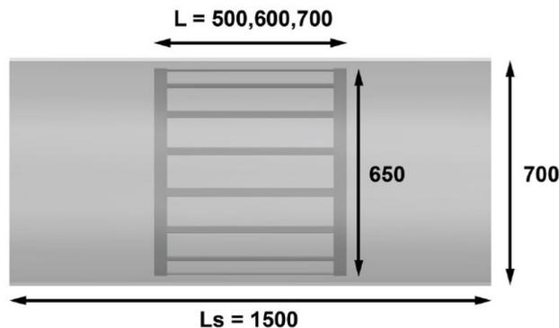
Figure 3: Physical dimensions of the cylindrical RF (birdcage) coils, HP\_B60\_Lz. All dimensions are provided in millimeters.
