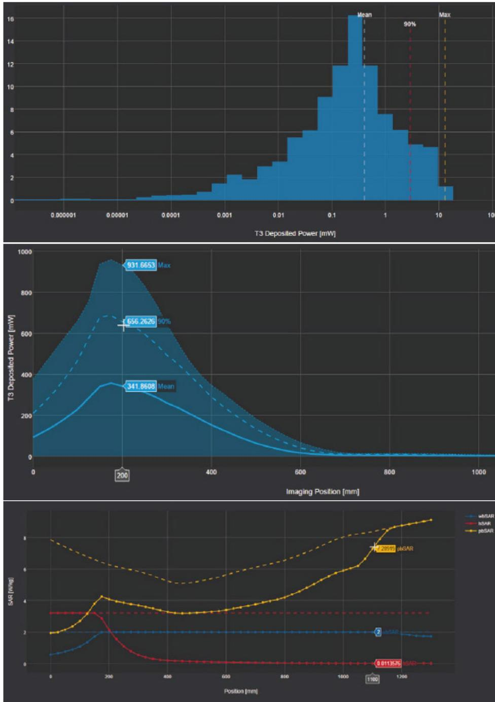
Figure 2: Example output of IMAalytics: histogram of deposited power (top), max/90%/mean statistics with respect to imaging position (middle), and corresponding whole-body SAR (wbSAR), head SAR (hSAR) and partial body SAR (pbSAR) values (bottom).
